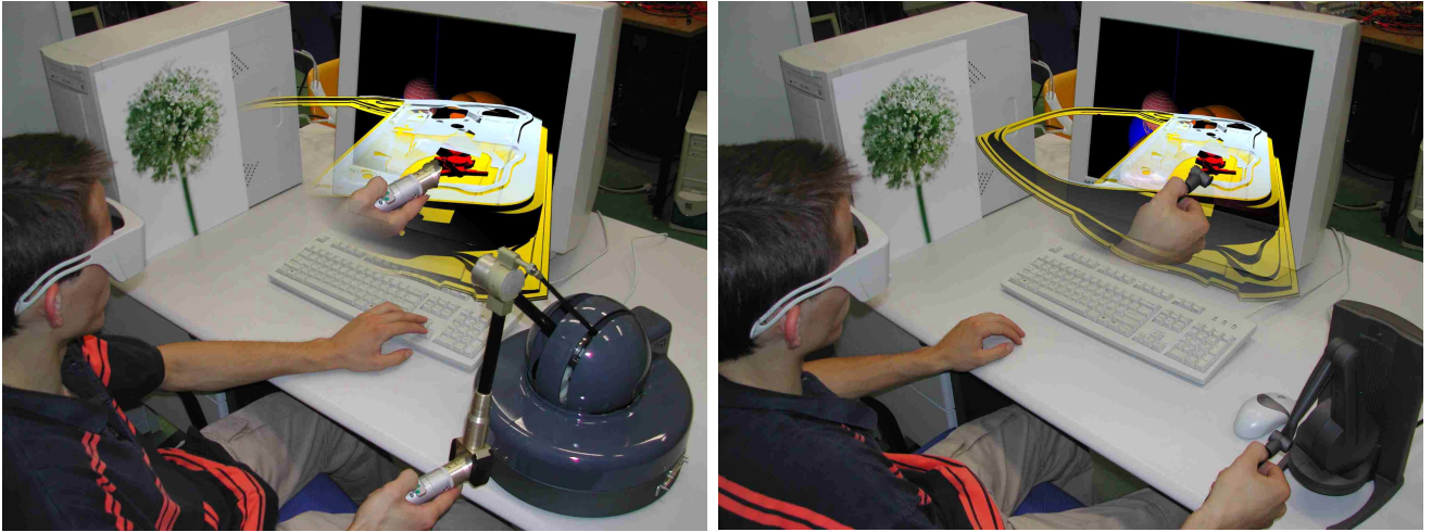
Fig. 6. Virtual prototyping application, the car door is a courtesy of RENAULT©. Left image show the scenario of a unmounting feasibility check with haptic feedback using the Virtuouse haptic device. The same image is illustrated right with the PHANTOM as a haptic device.
